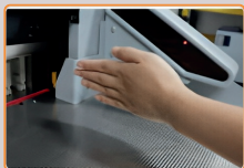
Six-way suspended photoelectric system for enhanced protection
