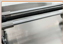
Ball screw + double guide rail. Cutting accuracy 0.2 mm
